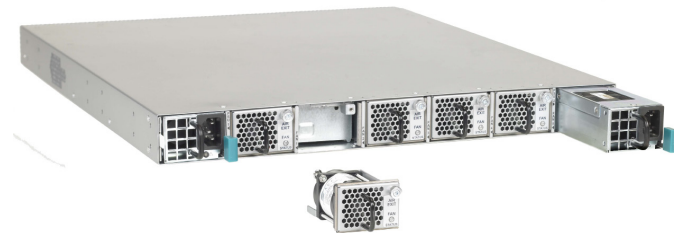
Arista 7048 Rear View : Redundant and hot-swappable fans and power supplies
