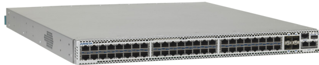
Arista 7048 Front View : 48-port 1000BASE-T (RJ-45) with 4 1/10GbE SFP+ uplinks
